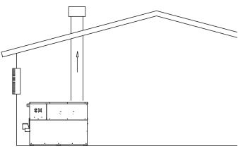
Figure 6 – Outside Combustion Air - Single Opening
